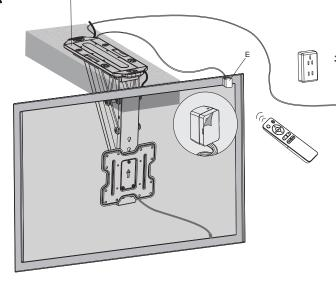
Do not plug into the power outlet until it is ready to be operated. Peel the backing paper. Place the IR receiver into desired position. Make sure nothing will obstruct the transmission from where the TV will be viewed.
