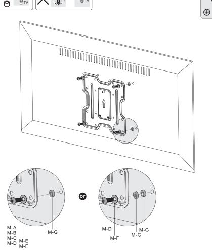
**Note:** Choose the appropriate screws, washers and spacers (if necessary) according to the type of screen. • Screw the VESA plate onto the TV.
