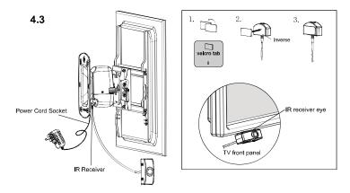
Plug the mount power cord into power outlet. Attach IR Receiver to TV: Using the provided Velcro tab, adhere the IR receiver eye-piece to the TV front panel so it has a clear line of sight with the remote control. (Fig. 6)
