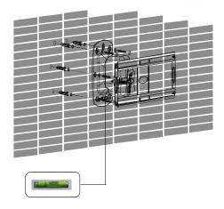
With the help of an assistant, and using the level to ensure the wall plate is level, position the wall plate against the wall in the desired mounting location.
