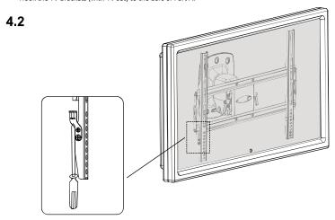
The lock designed feature can prevent your television from being removed from the crossbar. First, put the security lock in place, then tighten the bolt with screw driver by turning clockwise until tight (See illustration).
