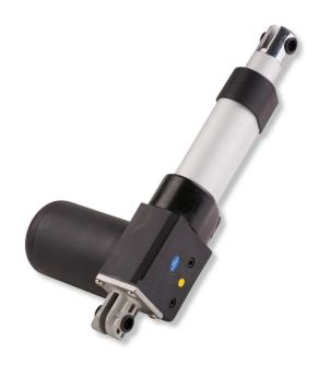
Deluxe Rod Linear Actuators are manufactured with a worm gear mechanism to provide quiet and fast operation. These durable and reliable actuators are available in various strokes and deliver 100 lbs. of force. With an extension rate of 3 inches per second the Deluxe Rod Actuator is our fastest actuator with 100 lb. of force.
