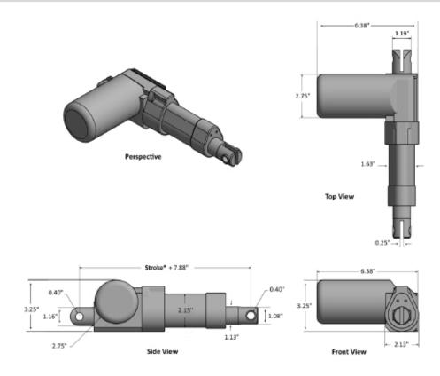
\*Stroke length tolerance ± 0.125"
