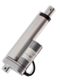
Classic Rod Linear Actuators are compact and versatile to suit the needs of a variety of automation projects. They are IP54 rated and manufactured with enhanced corrosion resistance to provide maximum life and value. Standard strokes up to 24 inches and forces up to 200 lbs are available as well as custom strokes and forces.
