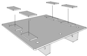
Place the VT Brackets (part #4) on the underside of the desktop. Carefully measure from all sides and attached the VT Brackets (part #4) to the underside of the desktop with thirty-two (32) Wood Screws (part #11), eight (8) per bracket.
