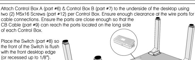
(or recessed up to 1/8"). The Switch may be placed anywhere along the front edge of the desktop but we recommend placing it toward an end so it does not interfere with the chairs when seated.
